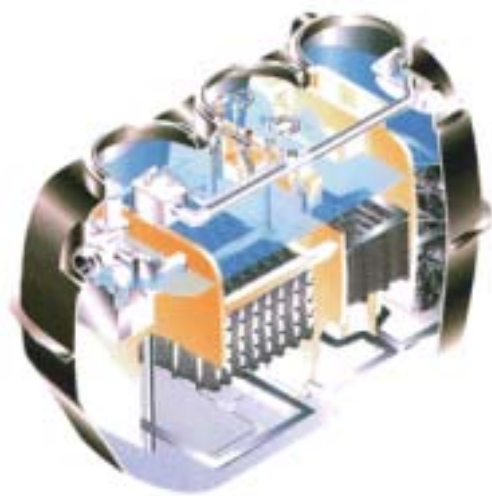
Fig.1 Structure of a small-scale johkasou system
